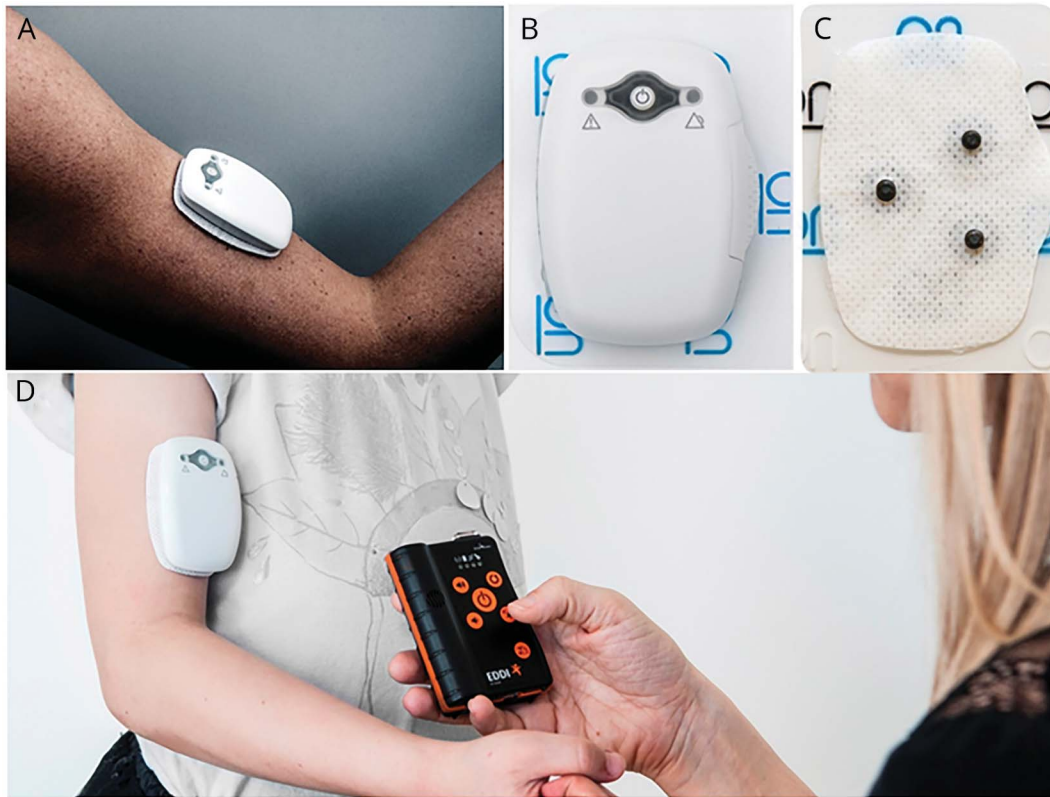
(A) The wearable device placed on the brachial biceps muscles. (B, C) The wearable device, which is connected to the self-adhesive patch, containing the recording electrodes and the ground electrode. (D) Remote control of the device.
